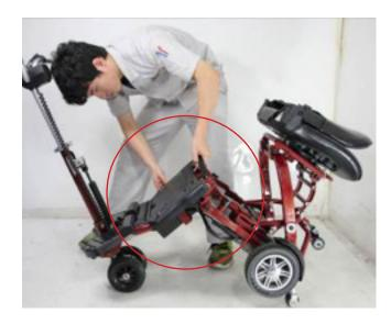
5. Push the tiller adjustment knob and fold the tiller.
