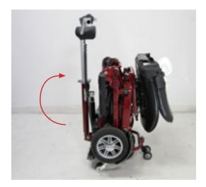
6. Loosen the tiller adjustment lever, fold down the tiller and re-tighten lever.
