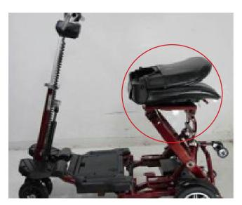
4. Pick up the frame separately with the handle bar and fold the rear frame.
