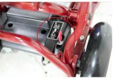
3. Pull the seat adjustment lever swivel seat towards the back of the scooter.
