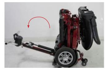
2. Pull the Separate Frame Safety Lever to unfold.
